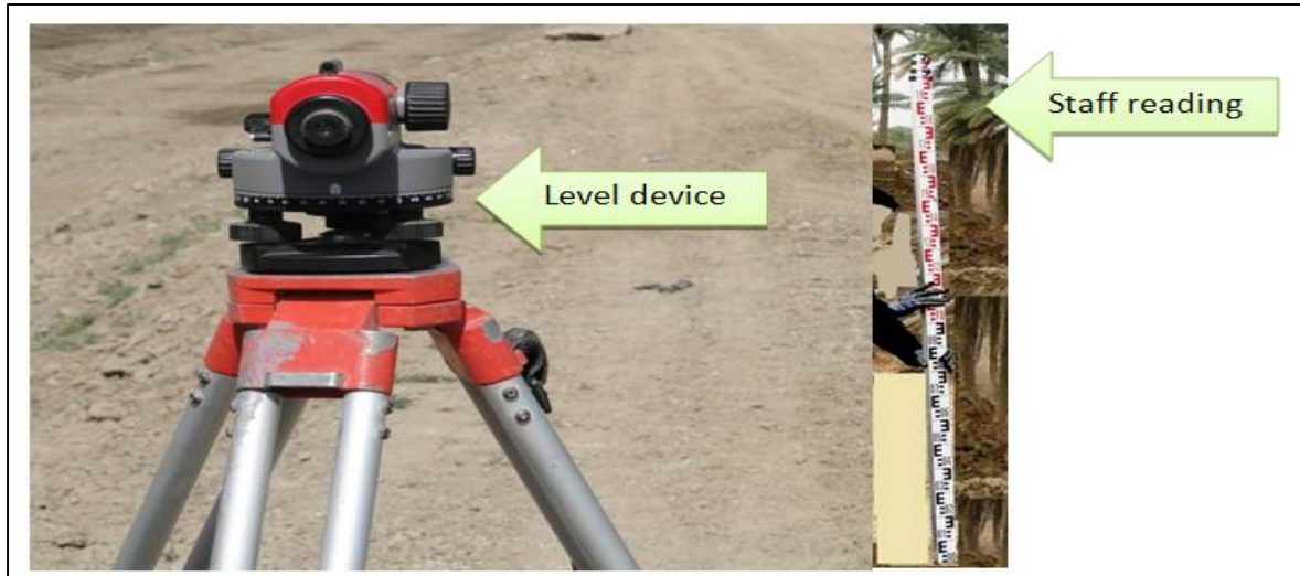
Figure (8) the image of level device with staff reading.
