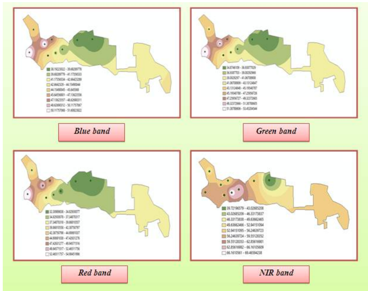
Figure 9: The interpolated data of the reflectance value of the water quality in Spring 2017 by using IDW interpolation over the AL-Hammar Marshes, South of Iraq.
